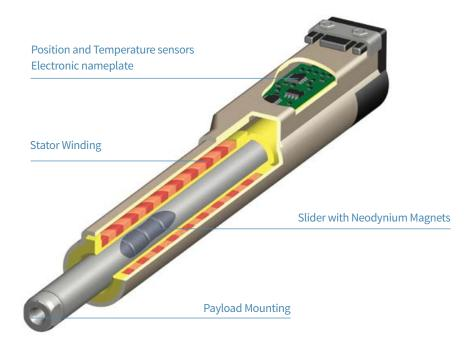
LinMot linear motors employ a direct electromagnetic principle. Electromagnetic force provides direct linear movement without the use of cams, gears, belts, or other mechanical devices. The engine consists of only two parts: The slider and the stator. The slider is made of neodymium magnets in a high precision stainless steel tube. In the stator are the motor windings, the bearing for the slider, the position detection and temperature sensors for thermal monitoring of the motor.
