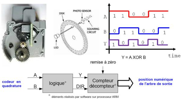
360 encoder pulses per revolution of a LEGO motor (1° resolution)with quadrature signals, (max resolution is 720 pulses/rev but not used)
