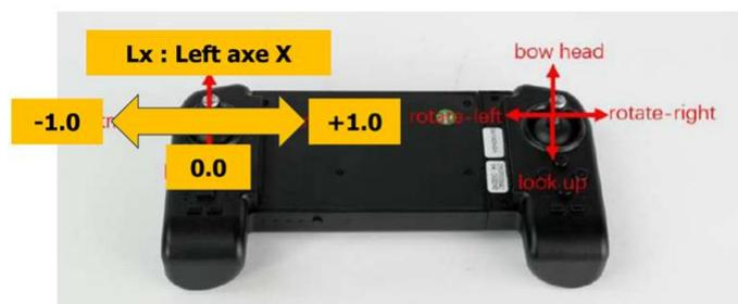
Figure 33 : Commande joystick Lx
