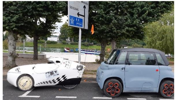
Figure 21 : Vélomobile (50kg, 3KW) et Citroën AMI (450kg, 5.8KW)
