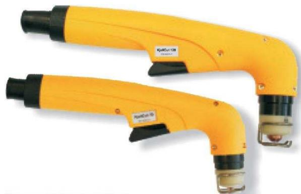
Plasma torch KjellCut 70 for CUTi 40 and CUTi 70 and KjellCut 120 for CUTi 90 and CUTi 120, both with a distance spring for keeping a constant distance to the workpiece and for observing the plasma arc.
