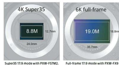
Super35 17:9 mode with PXW-FS7M2. Full-frame 17:9 mode with PXW-FX9
