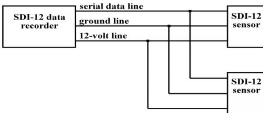
The asynchronous serial data line is a bidirectional (half-duplex) data transfer line.
