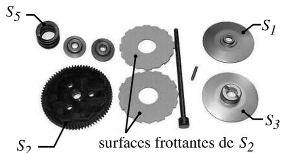
**Figure 23** - Éléments composant le " slipper "
