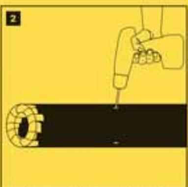
2 File down and pad the ends with foam and gaffer tape, and drill holes in both sides.
