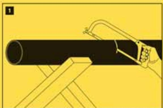
1 Use a hacksaw to cut the metal pipe into lengths of about 4 ft. shorter ones are possible, but make access to the 'cuffs' easier.
