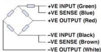
WIRING SCHEMATIC DIAGRAM
